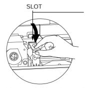
6. Replace Cartridge into printer. Make sure the arrow on top of the assembly is facing toward the rear of the printer. Hook assembly into slot on printer and rotate down. Ensure the assembly locks in place.
